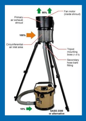
High Flow Biological Air sampling system based wet cyclone for extreme temperature -32°-+54°C
